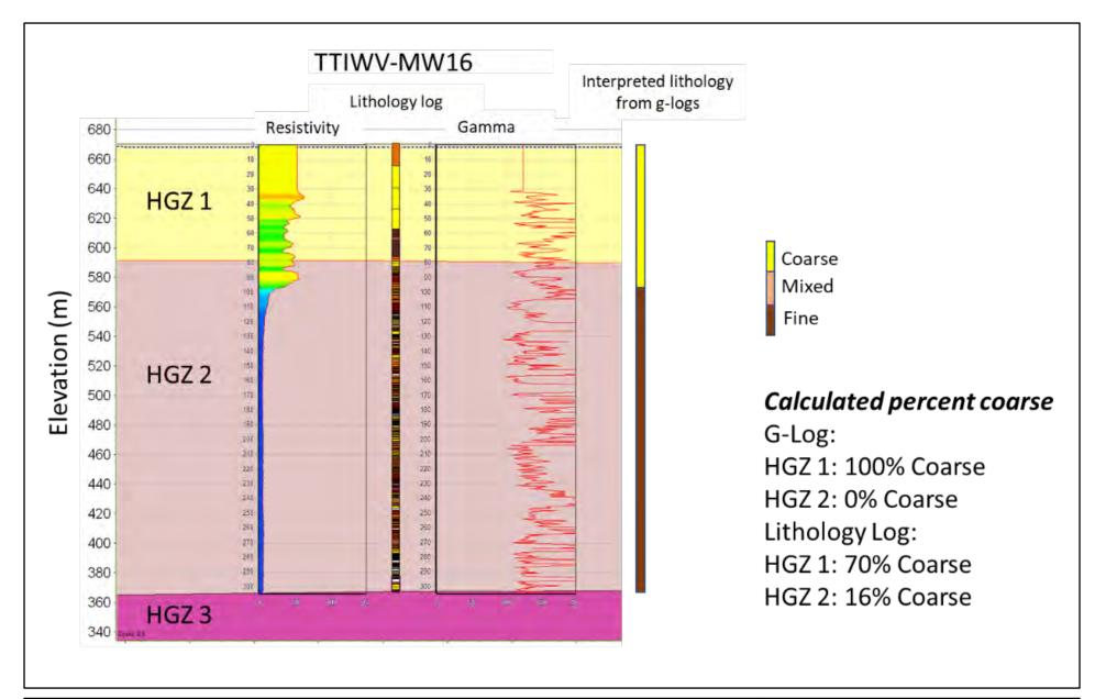
Note that the lithology log is more detailed and does not correspond fully with the resistivity and gamma log. Thus, the interpreted boundary between coarse and fine materials based on the geophysical log, shown on the right side of the figure, is lower than the interpretation from the lithology log.
